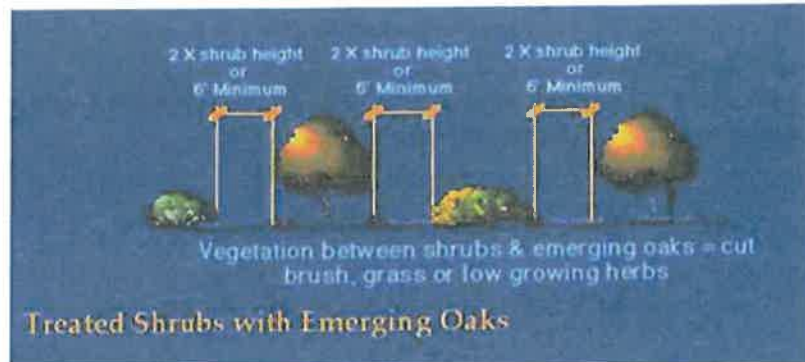
Figure 16. Shrub island spacing. Design groups of plants small enough to provide horizontal separation between groups. This allows proper maintenance and helps slow the spread of fire. Each shrub or group of plants should measure no wider than two times its height, or less than 120 sq. ft. (or 6 ft x 20 ft). The space between groups should be greater than three times the height of the shrubs, or at least a 12 ft. distance
