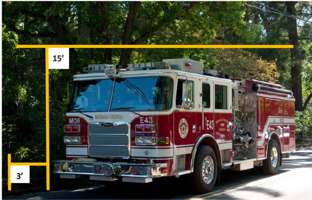
Cut Branches Overhanging the Roadway to Provide Clearance for the Fire Department Vehicles
